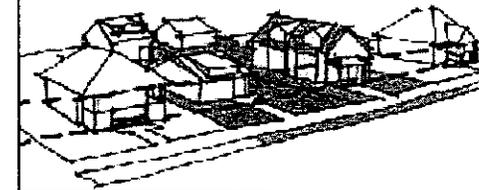
Dividing total building mass into separate structures is encouraged. The top illustration shows inappropriate massing while the bottom shows how building mass can be broken into separate elements.
